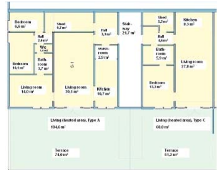
Plan for a large and a small apartment (showing two of four departments on the ground floor)
